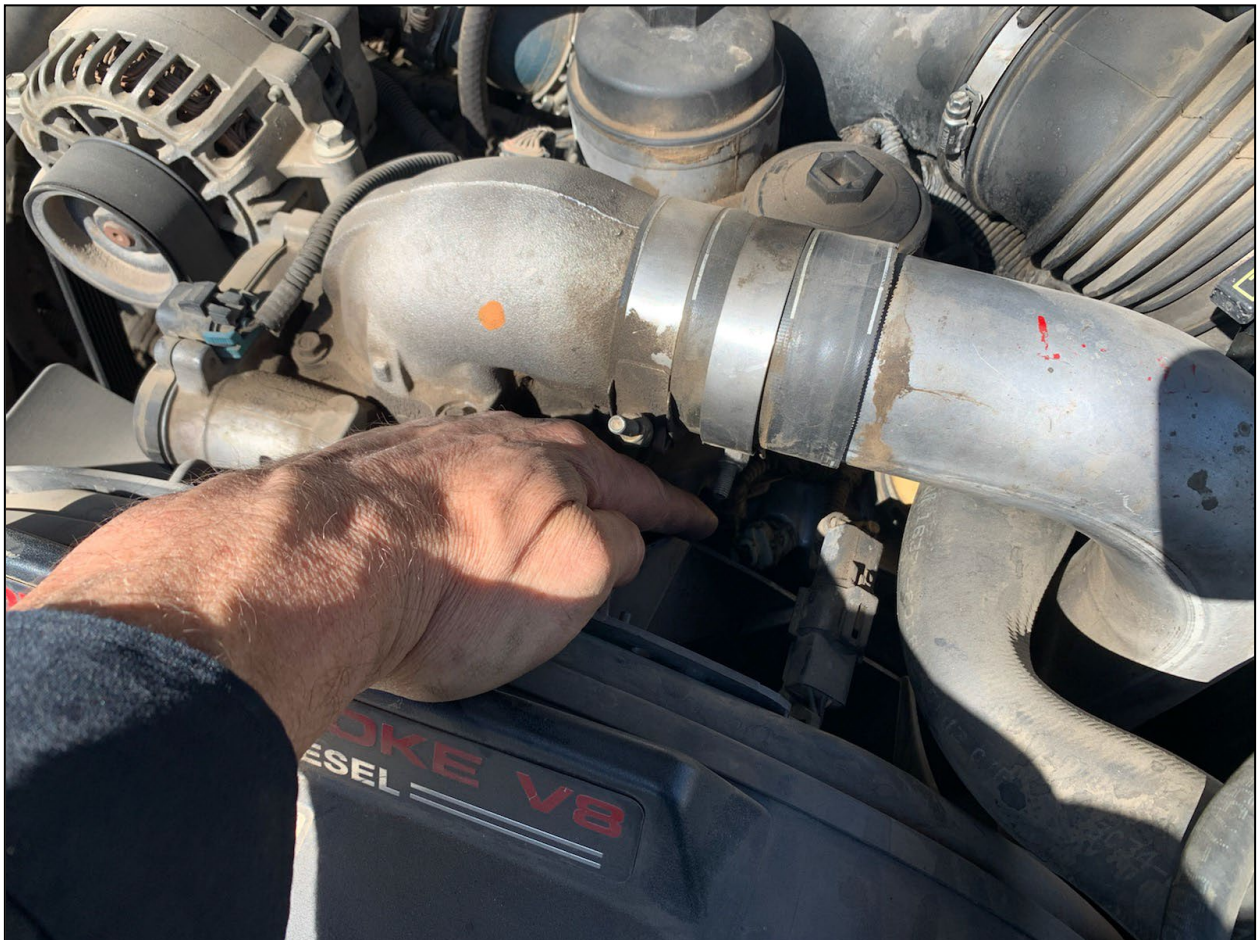
FIGURE 1 – POINTING AT COOLANT TEMPERATURE SENSOR
